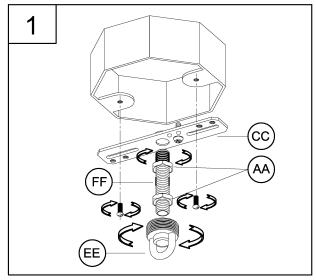
1. Install the chain holder (EE) onto the nipple (FF). Next, loosely thread the hex nuts (AA) onto the nipple (FF) and then thread this assembly onto the mounting plate (CC). Install this assembly to the outlet box using the mounting screws supplied with the outlet box (not included).
