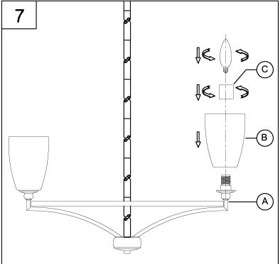
7. Attach the glass shades (B) to the fixture (A) using the socket rings (C) to secure them tightly.
