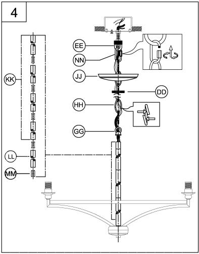
NOTE: During this step, determine the hanging length of your fixture by removing chain links (HH) and optionally cutting the electrical and ground wire to length.
