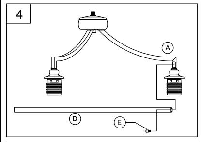
4. Attach the ring (D) to the fixture (A) using the studs (E) to secure it tightly.
