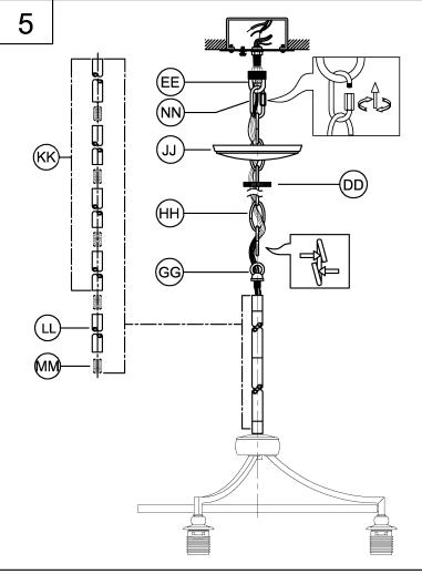
NOTE: During this step, determine the hanging length of your fixture by removing chain links (HH) and optionally cutting the electrical and ground wire to length.
