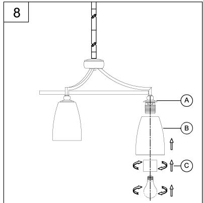
8. Attach the glass shades (B) to the fixture (A) using the socket rings (C) to secure them tightly.
