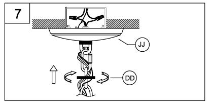
7. Tuck the wires into the junction box and slip the canopy (JJ) over the chain holder. Thread the screw collar (DD) onto the chain holder to secure the canopy tightly to the ceiling.
