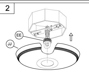
2. In this step, you will adjust the depth of the chain holder in relation to the canopy depth.
