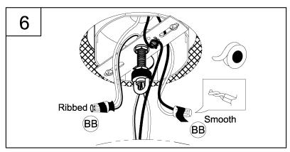
6. Strip 3/8" of insulation from the electrical wire ends. Using wire nuts (BB), connect the RIBBED fixture wire to the WHITE supply wire from the outlet box; connect the SMOOTH fixture wire to the BLACK supply wire.
