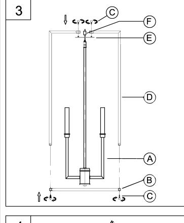
3. Pass the wires through the support plate (E) and coupling (F), attach the support plate (E) to the hang straight of fixture (A) use the coupling (F) to secure tightly. Then attach four rectangle tube (D) to the support plate (E) use screw (C) to secure tightly.
