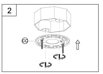
Next, take the fixture down and go back and tighten the hex nuts (DD) up against the mounting strap (CC). You now should have the correct length of threads for mounting the fixture.
