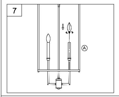
7. Thread the lamp (not included) into the fixture socket. Use 60-watt MAX incandescent candelabra base, SBCFL or SBLED.
