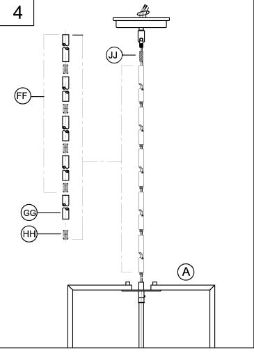
NOTE: During this step, determine the hanging length of your fixture by adding or removing stems. The electrical and ground wire may also optionally be cut to length.
