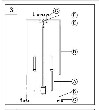
3. Pass the wires through the support plate (E) and coupling (F), attach the support plate (E) to the hang straight of fixture (A) use the coupling (F) to secure tightly.
