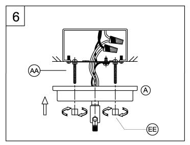
6. Pass the screws through the two holes in the canopy. Secure the fixture (A) to the screws (AA) using the two cylinder nuts (EE). Tighten securely.
