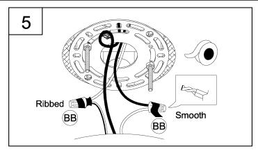
5. Strip 3/8" of insulation from the electrical wire ends. Using wire nuts (BB), connect RIBBED fixture wire to the WHITE supply wire from the outlet box; connect the SMOOTH fixture wire to the BLACK supply wire.
