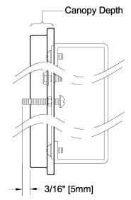
Thread both screws in or out for adjustment
