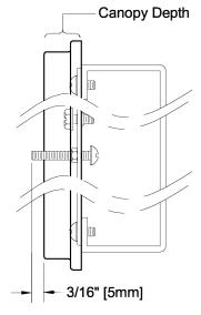
Thread both screws in or out for adjustment
