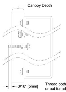
Thread both screws in or out for adjustment
