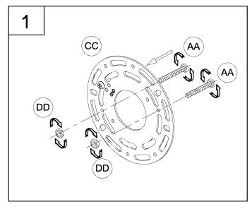
1. Loosely thread the screws (AA) and the hex nuts (DD) onto the round mounting plate (CC). You now need to adjust the screw length according to the fixture canopy depth.
