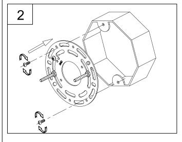
2. Attach assembled parts from Step 1 onto outlet box using the mounting screws supplied with the outlet box (not included).
