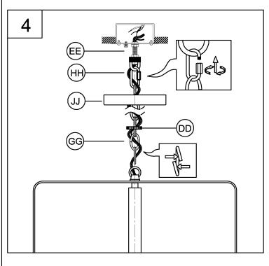
4. Weave wires through chain (GG) / quick link (HH). Pass wires and chain through screw collar (DD) and canopy (JJ). Open one link of chain and attach it to chain loop, close the chain link. And the other end lock to chain holder (EE) use quick link (HH) to secure tightly. Pass the wires through the chain holder/threaded nipple/ mounting plate.
