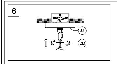
6. Tuck the wires into the outlet box and slip the canopy over the chain holder. Thread the screw collar (DD) onto the chain holder to secure the canopy tightly to the ceiling.
