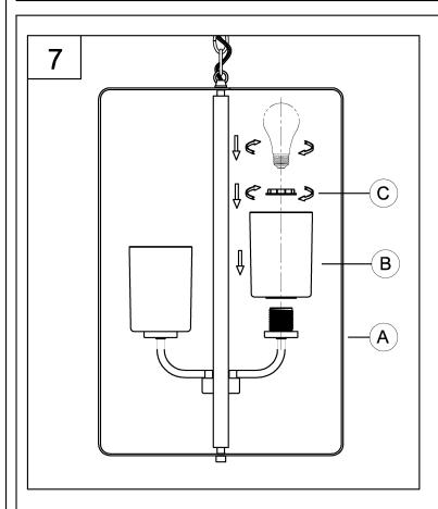
7. Place glass shades (B) onto fixture glass holders (A) use socket ring (C) to secure tightly.
