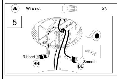
5. Strip 3/8" of insulation from the electrical wire ends. Using wire nuts (BB), connect RIBBED fixture wire to the WHITE supply wire from the outlet box; connect the SMOOTH fixture wire to the BLACK supply wire.
