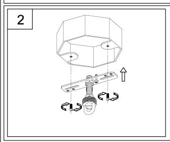
2. Attach assembled parts from Step 1 onto outlet box using the mounting screws supplied with the outlet box (not included).
