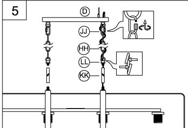
5. Pass the wire through the pipe (KK) \ chain loop (LL); Weave wires through chain (HH) / quick link (JJ) and canopy (D). Attach one end of pipe (KK) onto fixture (A) and other end to the chain loop (LL). Open one link of chain and attach it to chain loop, close the chain link. The other end lock to chain loop of canopy use quick link (JJ) to secure tightly.
