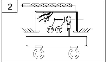
2. Use a drill with a #29 (Ø.136) (3.5mm) bit to create mounting holes in the outlet box.
