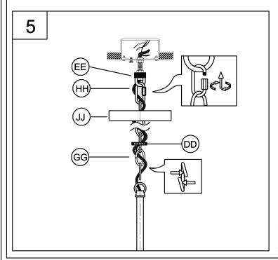
5. Weave wires through chain (GG) / quick link (HH). Pass wires and chain through screw collar (DD) and canopy (JJ). Open one link of chain and attach it to chain loop, close the chain link. And the other end lock to chain holder (EE) use quick link (HH) to secure tightly. Pass the wires through the chain holder/threaded nipple/mounting plate.
