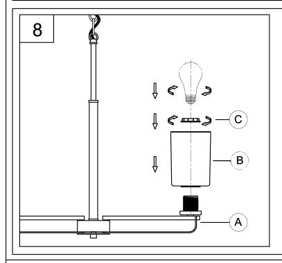
8. Place glass shades (B) onto fixture glass holders (A) use socket ring (C) to secure tightly.
