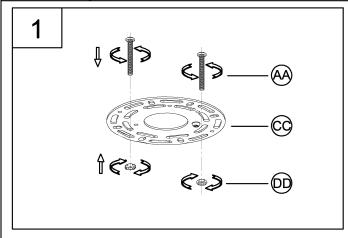
1. Screw screw (AA) onto round mounting plate (CC) and use hex nut (DD) to secure it tightly.
