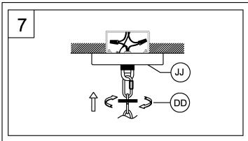
7. Tuck the wires into the outlet box and slip the canopy over the chain holder. Thread the screw collar (DD) onto the chain holder to secure the canopy tightly to the ceiling.
