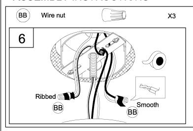
6. Strip 3/8" of insulation from the electrical wire ends. Using wire nuts (BB), connect RIBBED fixture wire to the WHITE supply wire from the outlet box; connect the SMOOTH fixture wire to the BLACK supply wire.
