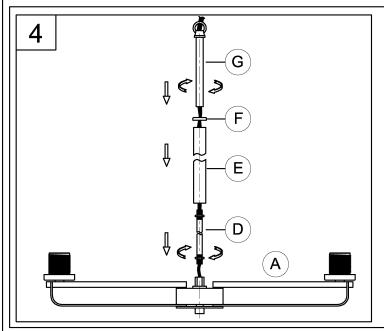
4. Pass the wires through the stem (D), tube (E), check ring (F), pipe (G). Then screw stem (D) into fixture (A), attach tube (E), check ring (F) on to stem (D), use pipe (G) to secure tightly.
