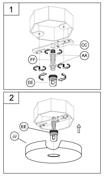
1. Install the chain holder (EE) onto the nipple (FF). Next, loosely thread the hex nuts (AA) onto the nipple (FF) and then thread this assembly onto the mounting strap (CC). Install this assembly to the outlet box using the mounting screws supplied with the outlet box (not included).
