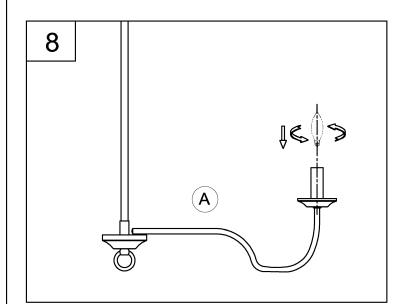
8. Thread the lamps (not included) into the fixture sockets. Use 60-watt MAX incandescent candelabra base, SBCFL or SBLED.
