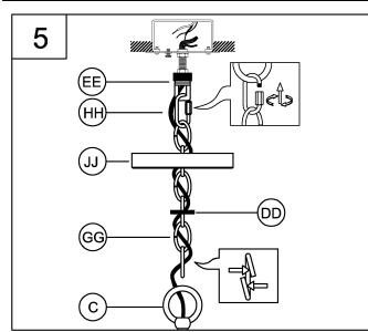
NOTE: During this step, determine the hanging length of your fixture by removing chain links (GG) and optionally cutting the electrical and ground wire to length.
