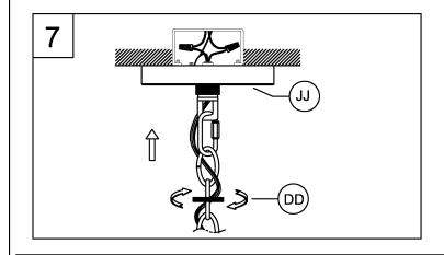
7. Tuck the wires into the outlet box and slip the canopy (JJ) over the chain holder. Thread the screw collar (DD) onto the chain holder to secure the canopy tightly to the ceiling.
