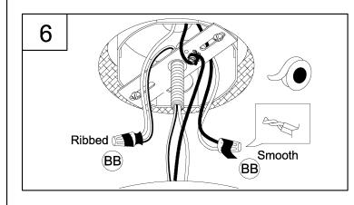
6. Strip 3/8" of insulation from the electrical wire ends. Using wire nuts (BB), connect the RIBBED fixture wire to the WHITE supply wire from the outlet box; connect the SMOOTH fixture wire to the BLACK supply wire. Connect the fixture ground wire and supply ground wire using a wire nut or by fastening to the ground screw on the mounting strap. Push all wire connections into the outlet box.
