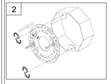
Attach assembled parts from Step 1 onto outlet box using the mounting screws supplied with the outlet box (not included).
