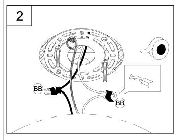
2. Strip 3/8" of insulation from the electrical wire ends. Using wire nuts (BB), connect white fixture wire to the white supply wire from the outlet box; connect the black fixture wire to the black supply wire.
