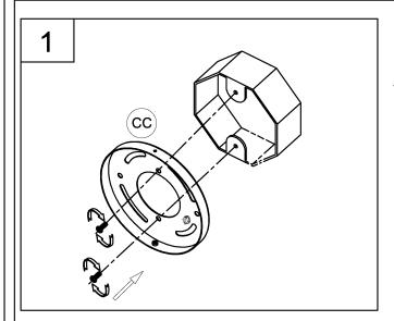
1. Attach round back plate (CC) to the outlet box and using the mounting screws to secure it tight (not included).
