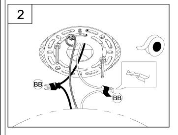
2. Strip 3/8" of insulation from the electrical wire ends. Using wire nuts (BB), connect white fixture wire to the white supply wire from the outlet box; connect the black fixture wire to the black supply wire.
