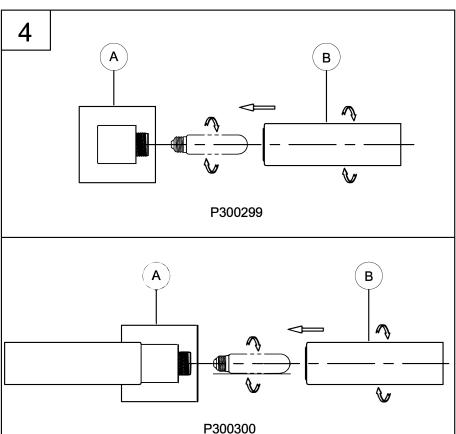
4. Screw lamp (not included) into fixture socket. Use 60-watt MAX incandescent medium base T lamp.
