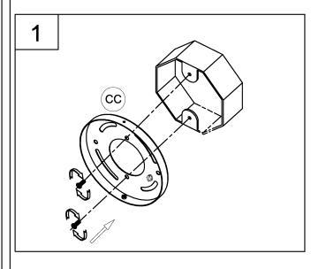
1. Attach round back plate (CC) to the outlet box and using the mounting screws to secure it tight (not included).
