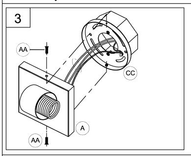
3. Attach fixture (A) to the round back plate (CC) and use screw (AA) to secure tight.
