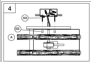
4. Attach fixture (A) to screws (AA) using cylinder nuts (EE). Secure tightly.
