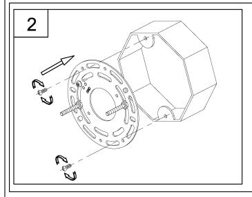
2. Attach assembled parts from Step 1 onto junction box, using the mounting screws supplied with the junction box (not included).
