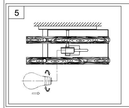
5. Screw two lamps (not included) into fixture sockets. Use 75-watt MAX incandescent medium base lamp, SBCFL or SBLED.
