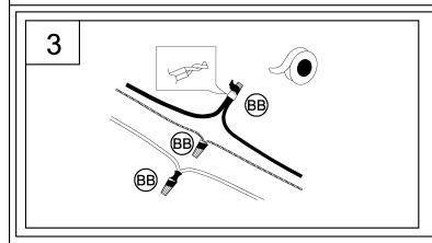
3. Strip 3/8" of insulation from the electrical wire ends. Using wire nuts (BB), connect white fixture wire to the white supply wire from the junction box; connect the black fixture wire to the black supply wire.
