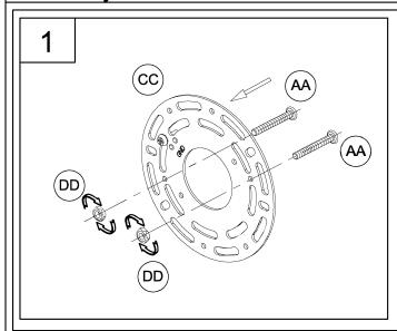
1. Screw screw (AA) onto Round mounting plate (CC) and use hex nut (DD) to secure it tight.
