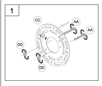
1. Loosely thread the screws (AA) and the hex nuts (DD) onto the the round mounting plate (CC).
