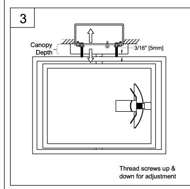
3. You now need to adjust the screw length (AA) according to the fixture canopy depth.
