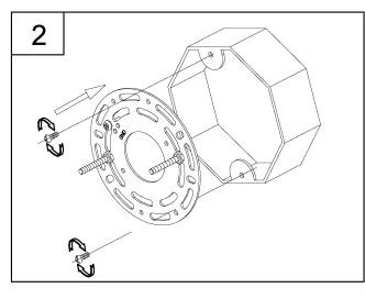
2. Attach this assembly to the outlet box using the mounting screws supplied with the outlet box (not provided). Tighten securely.
