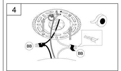
4. Strip 3/8" of insulation from the electrical wire ends. Using wire nuts (BB), connect the WHITE fixture wire to the WHITE supply wire from the outlet box; connect the BLACK fixture wire to the BLACK supply wire from the outlet box.
