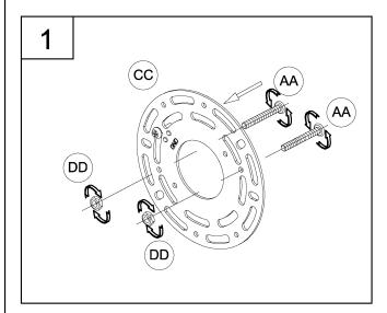
1. Loosely thread the screws (AA) and the hex nuts (DD) onto the the round mounting plate (CC).
