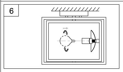
6. Screw lamp (not included) into fixture socket. Use 60-watt MAX incandescent candelabra base lamp, SBCFL or SBLED.
