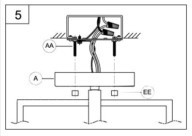
5. Slide the mounting holes in the fixture (A) over the screws (AA) and using the cylinder nuts (EE), tighten the fixture against the ceiling surface.
