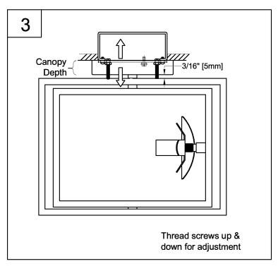
3. You now need to adjust the screw length (AA) according to the fixture canopy depth.
