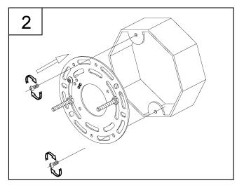
2. Attach this assembly to the outlet box using the mounting screws supplied with the outlet box (not provided). Tighten securely.
