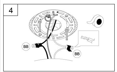
4. Strip 3/8" of insulation from the electrical wire ends. Using wire nuts (BB), connect the WHITE fixture wire to the WHITE supply wire from the outlet box; connect the BLACK fixture wire to the BLACK supply wire from the outlet box.
