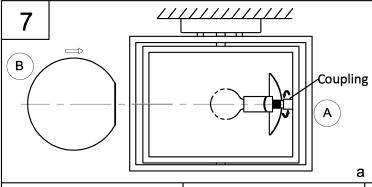
7. Attach glass shade (B) to fixture (A) and using coupling to secure tightly.
