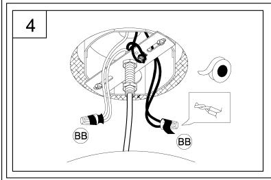
4. Strip 3/8" of insulation from the electrical wire ends. Using wire nuts (BB), connect white fixture wire to the white supply wire from the outlet box; connect the black fixture wire to the black supply wire.
