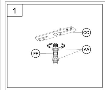
1. Screw threaded nipple (FF) into mounting strap (CC) several turns. Use one hex nut (AA) to secure parts tightly. Screw one hex nut (AA) onto threaded nipple (FF).
