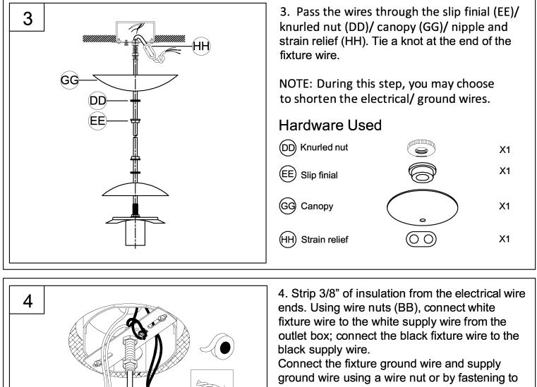
the ground screw on the mounting strap. Push all wire connections into the outlet box.
