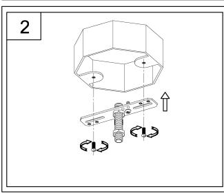
2. Attach assembled parts from Step 1 onto outlet box using the mounting screws supplied with the outlet box (not included).
