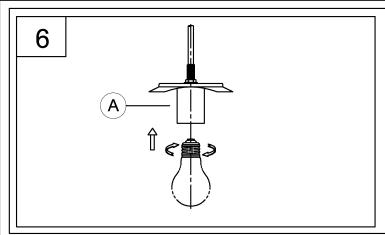
6. Screw lamp (not included) into fixture socket (A). Use 60-watt MAX incandescent medium base lamp, SBCFL or SBLED.
