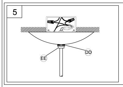
5. Tuck the wires into the outlet box and slip the canopy over the nipple. Thread the slip finial (EE) and knurled nut (DD) on the nipple to secure the canopy tightly to the ceiling.
