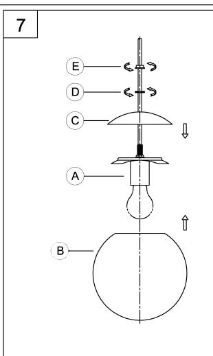
7. Attach glass globe (B) to fixture. Place glass cover (C) to fixture using knurled nut (D) and slip finial (E) to secure tightly.
