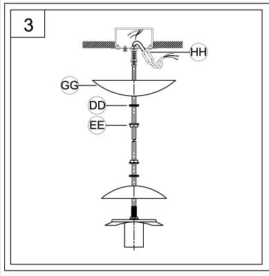
3. Pass the wires through the slip finial (EE)/knurled nut (DD)/canopy (GG)/ nipple and strain relief (HH). Tie a knot at the end of the fixture wire.
