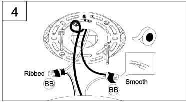
4. Strip 3/8" of insulation from the electrical wire ends. Using wire nuts (BB), connect RIBBED fixture wire to the WHITE supply wire from the outlet box; connect the SMOOTH fixture wire to the BLACK supply wire.
