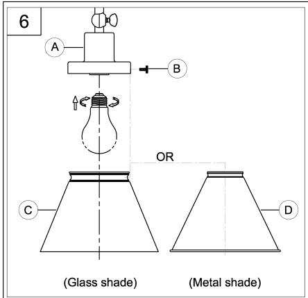
6. Screw lamp (not included) into the fixture socket. Use 100-watt MAX medium base lamp, SBCFL or SBLED.
