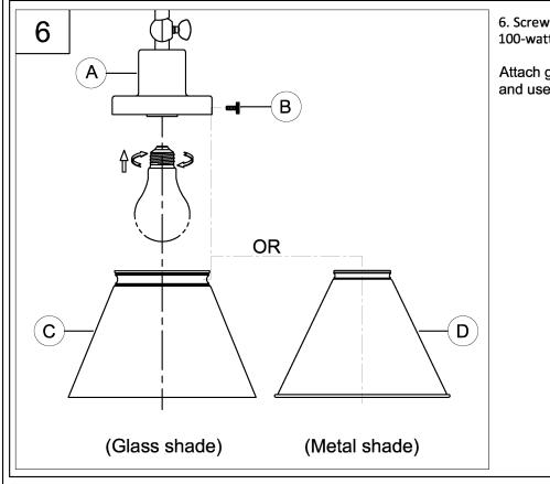
6. Screw lamp (not included) into the fixture socket. Use 100-watt MAX medium base lamp, SBCFL or SBLED.
