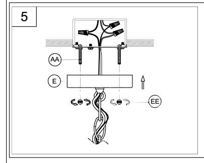
5. Secure the canopy (E) to screws (AA) use the ball nut (EE) to secure tightly.
