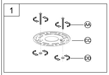
1. Screw screw (AA) onto round mounting plate (CC) and use hex nut (DD) to secure it tightly.
