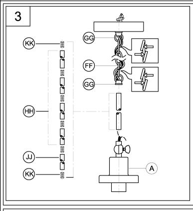
3. Pass the wires through the one pipe (JJ)/nipple (KK)/four pipes (HH) and chain loop (GG) to achieve overall desired length.
