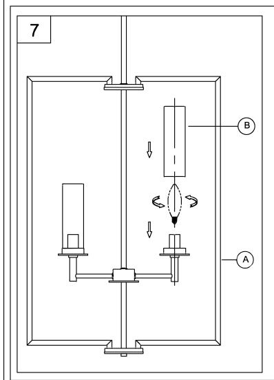
7. Screw lamp (not included) into fixture socket. Use 60-watt MAX incandescent candelabra base, SBCFL or SBLED.
