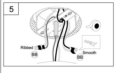
5. Strip 3/8" of insulation from the electrical wire ends. Using wire nuts (BB), connect RIBBED fixture wire to the WHITE supply wire from the outlet box; connect the SMOOTH fixture wire to the BLACK supply wire. Connect the fixture ground wire and supply ground wire using a wire nut or by fastening to the ground screw on the 1/8IP mounting plate. Push all wire connections into the outlet box.
