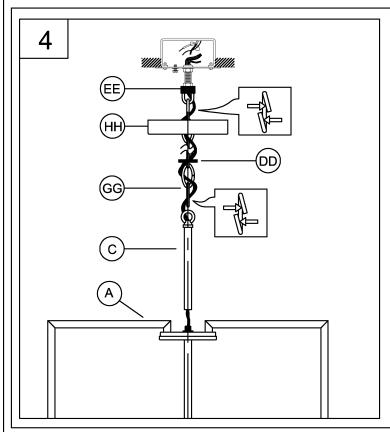
4. Pass the wires through the stem (C), than attach stem (C) onto fixture (A) to secure tightly. Weave wires through chain (GG). Pass wires and chain through screw collar (DD) and canopy (HH). Open two links of chain and attach one end to stem (C) and the other end to chain holder (EE). Close the chain links. Pass the wires through the chain holder/ threaded nipple/ mounting plate.
