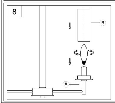
8. Screw lamp (not included) into fixture socket (A). Use 60-watt MAX incandescent candelabra base, SBCFL or SBLED.
