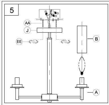
5. Attach fixture (A) to screws (AA) use cylinder nuts (EE) to Secure tightly.
