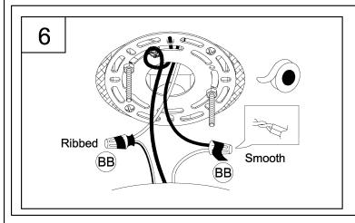
6. Strip 3/8" of insulation from the electrical wire ends. Using wire nuts (BB), connect RIBBED fixture wire to the WHITE supply wire from the outlet box; connect the SMOOTH fixture wire to the BLACK supply wire.
