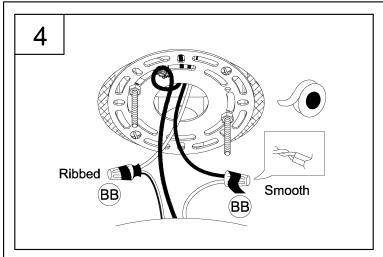
4. Strip 3/8" of insulation from the electrical wire ends. Using wire nuts (BB), connect RIBBED fixture wire to the WHITE supply wire from the outlet box; connect the SMOOTH fixture wire to the BLACK supply wire.
