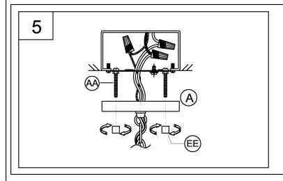
5. Secure the canopy to screws (AA) using the two cylinder nuts (EE). Tighten securely.
