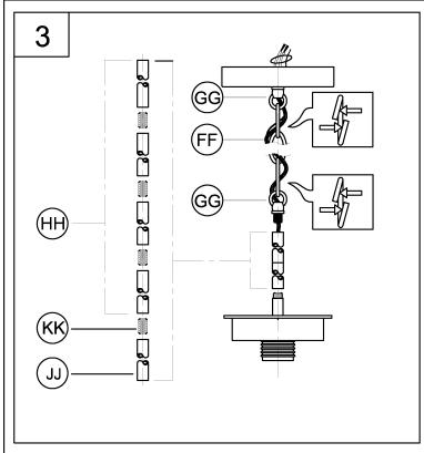
3. Pass the wires through the nipple (KK)/one pipe (JJ)/ four pipe (HH) to achieve overall desired length. Next attach pipe onto fixture using nipple (KK). Secure tightly.
