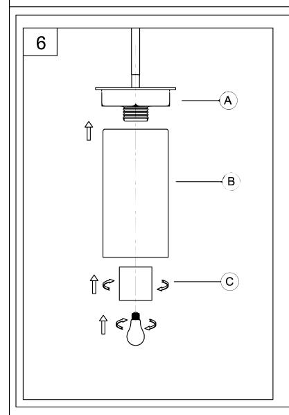
6. Place glass shade (B) into fixture (A) using socket ring (C) to secure it tightly. Screw lamp (not included) into fixture socket. Use 60-watt MAX incandescent medium base lamp, SBCFL or SBLED.
