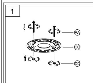
1. Screw screw (AA) onto round mounting plate (CC) and use hex nut (DD) to secure it tightly.
