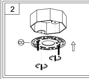
2. Attach assembled parts from step 1 onto outlet box, using the mounting screws supplied with the outlet box (not included).
