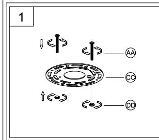
1. Screw screw (AA) onto round mounting plate (CC) and use hex nut (DD) to secure it tightly.
