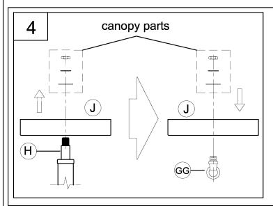
4. Remove existing canopy parts and canopy (J) from coupling (H).
