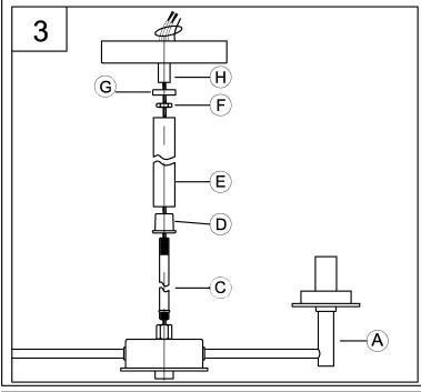
3. Pass the wires through the stem (C)/ seat ring (D) and round tube (E). Screw stem (C) into fixture (A). Attach seat ring (D) and round tube (E) onto stem (C). Pass the wires through the hex nut (F)/seat ring (G)/ coupling (H). Screw hex nut (F) onto stem (C), attach seat ring (G)/ coupling (H) onto stem (C) secure them tightly.
