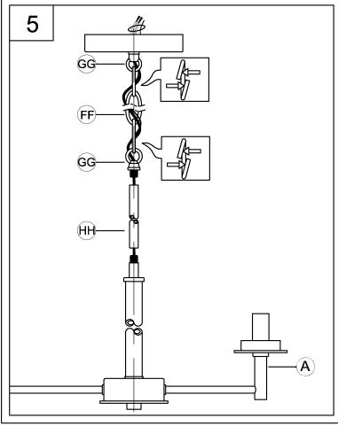
5. Pass the wires through pipe (HH) / chain loop (GG). attach chain loop (GG) to fixture (A) use pipe (HH) to secure tightly.
