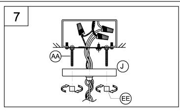
7. Secure the canopy (J) to screws (AA) use the two cylinder nuts (EE). Tighten securely.
