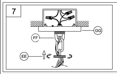
7. Slip the canopy (GG) over the chain holder (FF) Thread the screw collar (EE) onto the chain holder to secure the canopy tightly to the ceiling.
