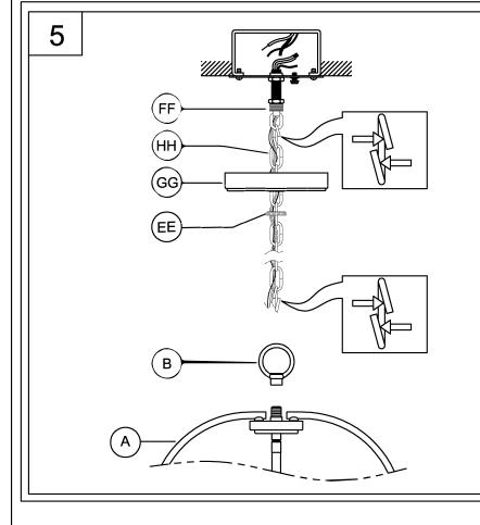
5. Pass the wires through the chain loop (B) and secure tightly onto fixture (A). Weave wires through chain (HH). Pass wires through screw collar (EE) and canopy (GG). Open two links of chain and attach one end to chain loop (B) and the other end to the chain holder (FF). Close the chain links. Pass the wires through the chain holder/threaded nipple/crossbar.
