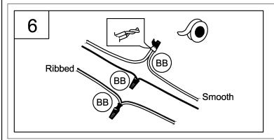
6. Strip 3/8" of insulation from the electrical wire ends. Using wire nuts (BB), connect RIBBED fixture wire to the WHITE supply wire from the outlet box; connect the SMOOTH fixture wire to the BLACK supply wire.
