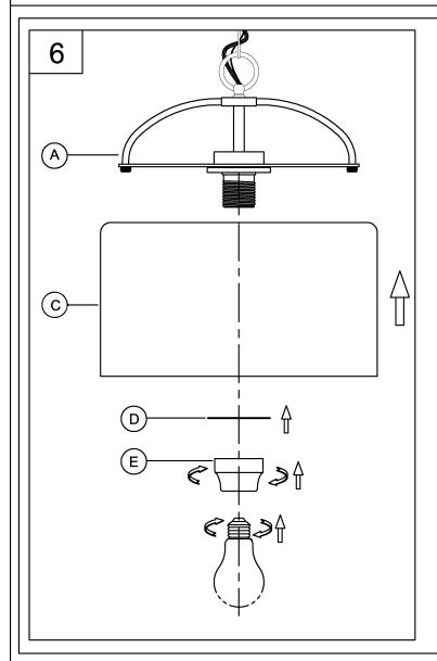
6. Attach glass shade (C) to fixture (A) using steel washer (D) and socket ring (E) to secure it tightly.
