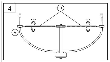
4. Attach tube (D) to fixture (A) and secure tightly.
