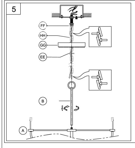
5. Pass the wires through the stem (B) and secure tightly onto fixture (A). Weave wires through chain (HH). Pass wires through screw collar (EE) and canopy (GG). Open two links of chain and attach one end to stem (B) and the other end to the chain holder (FF). Close the chain links. Pass the wires through the chain holder/ threaded nipple/crossbar.
