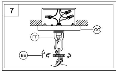
7. Slip the canopy (GG) over the chain holder (FF) Thread the screw collar (EE) onto the chain holder to secure the canopy tightly to the ceiling.
