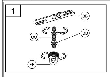
1. Screw threaded nipple (CC) into mounting strap (BB) several turns. Use one hex nut (DD) to secure parts tightly. Thread one hex nut (DD) and chain holder (FF) onto threaded nipple (CC). Tighten the hex nut against the top of the screw collar loop.
