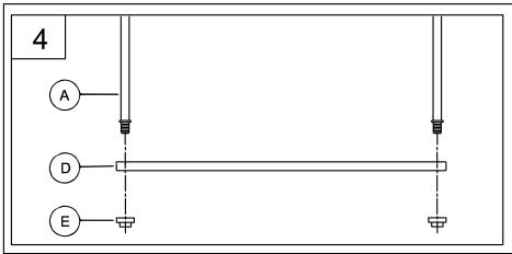
4. Attach flat tube ring (D) to fixture (A), using finial (E) to secure tightly.
