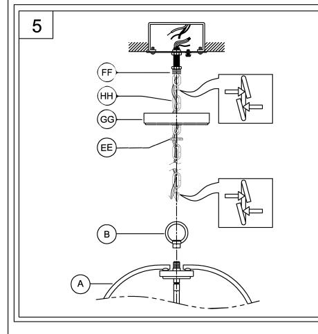
5. Pass the wires through the chain loop (B) and secure tightly onto fixture (A). Weave wires through chain (HH). Pass wires screw collar (EE) and canopy (GG). Open two links of chain and attach one end to chain loop (B) and the other end to the chain holder (FF). Close the chain links. Pass the wires through the / threaded nipple/crossbar.
