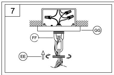
7. Slip the canopy (GG) over the chain holder (FF) Thread the screw collar (EE) onto the chain holder to secure the canopy tightly to the ceiling.
