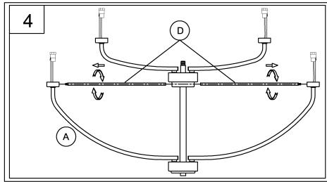
4. Attach tube (D) to fixture (A) and secure tightly.
