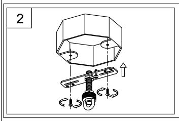
2. Attach assembled parts from step 1 onto outlet box using the mounting screws supplied with the outlet box (not included).
