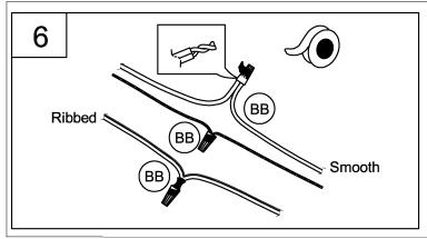
6. Strip 3/8" of insulation from the electrical wire ends. Using wire nuts (BB), connect RIBBED fixture wire to the WHITE supply wire from the outlet box; connect the SMOOTH fixture wire to the BLACK supply wire.
