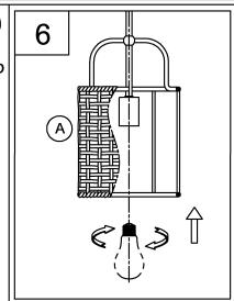
6. Screw lamp (not included) into fixture socket. Use 60-watt MAX incandescent medium base lamp, SBCFL or SBLED.
