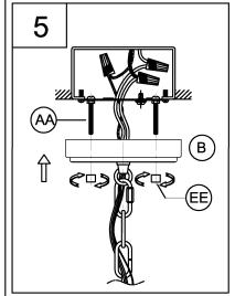
5. Secure the canopy (B) to screws (AA) use the two cylinder nuts (EE) to secure tightly.
