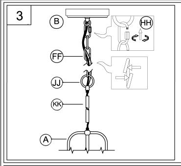
3. Pass the wires through the pipe (KK) and chain loop (JJ). Attach the pipe (KK) onto fixture (A) to secure it tightly. Next Weave electric cord and ground wire through chain (FF). Open one link of chain and attach this end to chain loop (JJ). Close the chain link. Attach the other end of chain link (FF) to canopy loop (B) using quick-link (HH) to secure it tightly.
