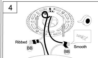
4. Strip 3/8" of insulation from the electrical wire ends. Using wire nuts (BB), connect RIBBED fixture wire to the WHITE supply wire from the outlet box; connect the SMOOTH fixture wire to the BLACK supply wire. Connect the fixture ground wire and supply ground wire using a wire nut or by fastening to the ground screw on the round mounting plate. Push all wire connections into the outlet box.
