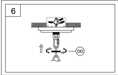
6. Tuck the wires into the outlet box and slip the canopy over the chain holder. Thread the screw collar (DD) onto the chain holder to secure the canopy tightly to the ceiling.
