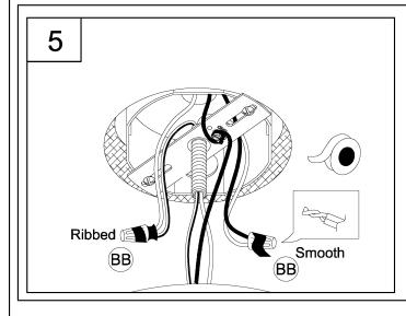
5. Strip 3/8" of insulation from the electrical wire ends. Using wire nuts (BB), connect RIBBED fixture wire to the WHITE supply wire from the outlet box; connect the SMOOTH fixture wire to the BLACK supply wire. Connect the fixture ground wire and supply ground wire using a wire nut or by fastening to the ground screw on the mounting plate. Push all wire connections into the outlet box.
