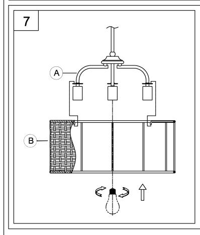
7. Place wicker shade (B) onto fixture (A). Screw lamps (not included) into fixture socket. Use 60-watt MAX incandescent medium base lamp, SBCFL or SBLED.
