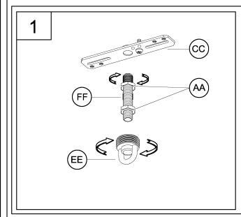
1. Screw threaded nipple (FF) into mounting plate (CC) several turns. Use one hex nut (AA) to secure parts tightly. Screw one hex nut (AA) and chain holder (EE) onto threaded nipple (FF). Tighten the hex nut against the top of the chain holder.
