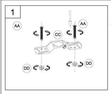
1. Screw screw (AA) onto mounting strap (CC) and use hex nut (DD) to secure it tight.
