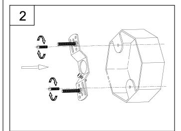
2. Attach assembled parts from step 1 onto outlet box using the mounting screws supplied with the outlet box (not included).
