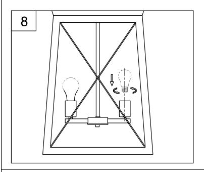
8. Thread the lamps (not included) into the fixture sockets. Use 60-watt MAX incandescent medium base lamp, SBCFL or SBLED.
