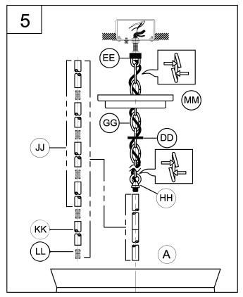
NOTE: During this step, determine the hanging length of your fixture by adding or removing pipes and chain links. The electrical and ground wire may also optionally be cut to length.
