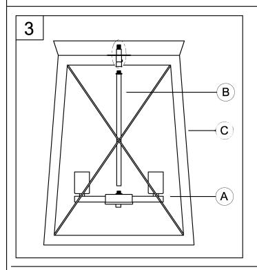
4. Attach fixture (A) to the metal frame (C) and use the stem (B) to secure it tightly.
