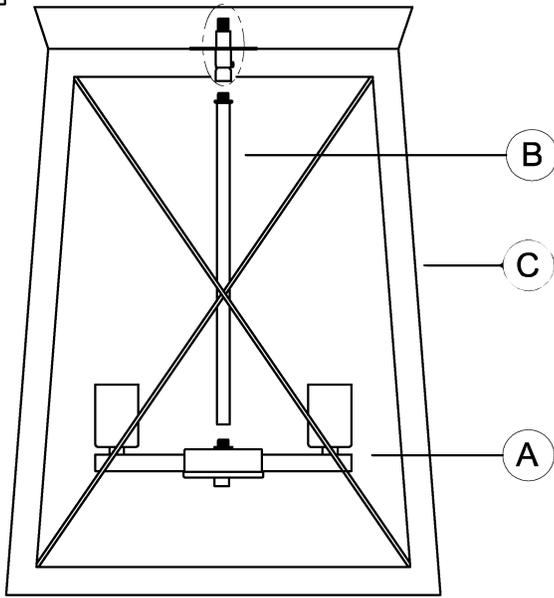
4. Attach fixture (A) to the metal frame (C) and use the stem (B) to secure it tightly.
