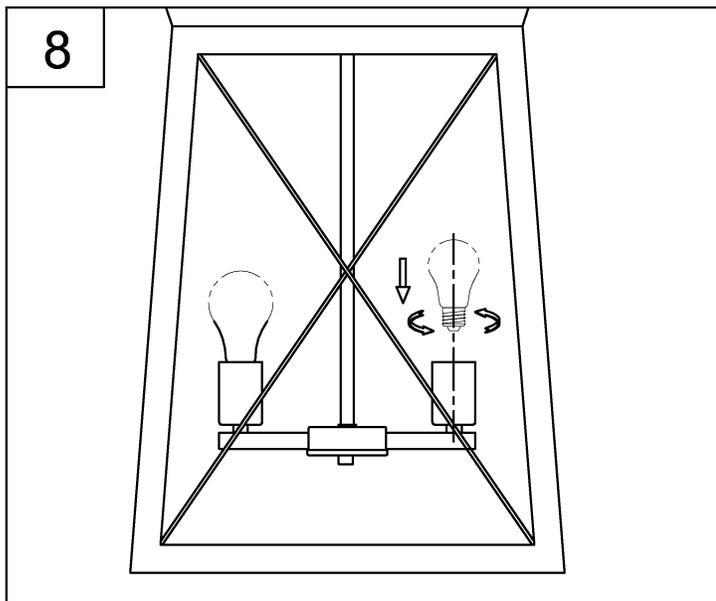
8. Thread the lamps (not included) into the fixture sockets. Use 60-watt MAX incandescent medium base lamp, SBCFL or SBLED.
