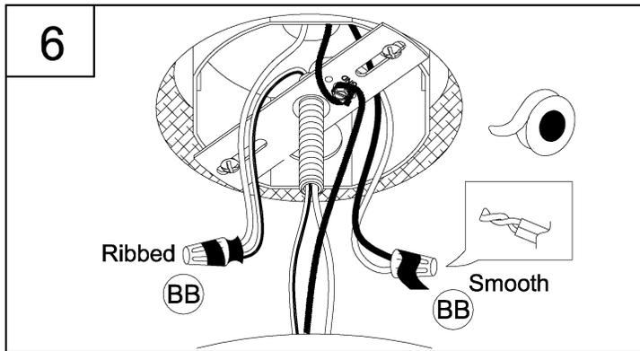
6. Strip 3/8" of insulation from the electrical wire ends. Using wire nuts (BB), connect the RIBBED fixture wire to the WHITE supply wire from the outlet box; connect the SMOOTH fixture wire to the BLACK supply wire. Connect the fixture ground wire and supply ground wire using a wire nut or by fastening to the ground screw on the mounting strap. Push all wire connections into the outlet box.
