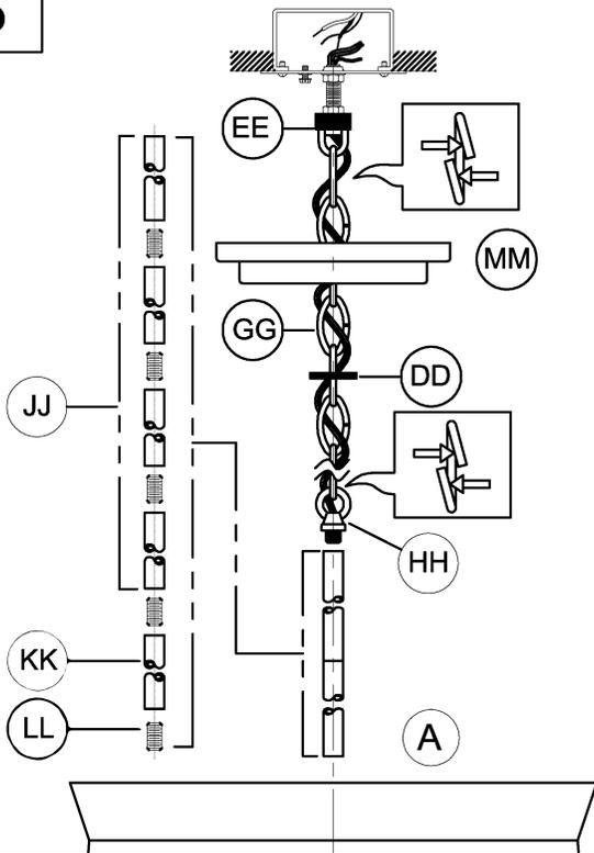
NOTE: During this step, determine the hanging length of your fixture by adding or removing pipes and chain links. The electrical and ground wire may also optionally be cut to length.
