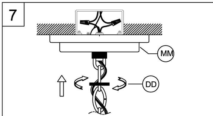
7. Tuck the wires into the outlet box and slip the canopy (MM) over the chain holder. Thread the screw collar (DD) onto the chain holder to secure the canopy tightly to the ceiling.
