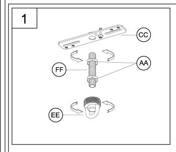
1. Screw threaded nipple (FF) into 1/8IP mounting strap (CC) several turns. Use one hex nut (AA) to secure parts tightly. Screw one hex nut (AA) and chain holder (EE) onto threaded nipple (FF). Tighten the hex nut against the top of the chain holder.
