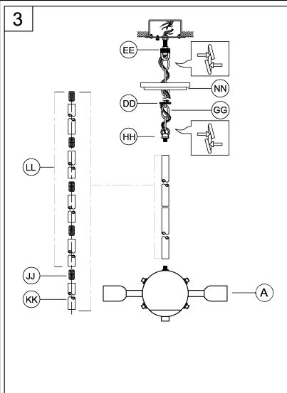
3. Pass the wires through the one pipe (KK)/nipple (JJ)/four pipe (LL) to achieve overall desired length. Screw pip (KK/LL) onto fixture (A). Pass the wires through the Chain loop (HH). Weave wires through chain (GG). Pass wires and chain through screw collar (DD) and canopy (NN). Open two links of chain and attach one end to chain loop (HH) and the other end to chain holder (EE). Close the chain links. Pass the wires through the chain holder/threaded nipple/ mounting strap.
